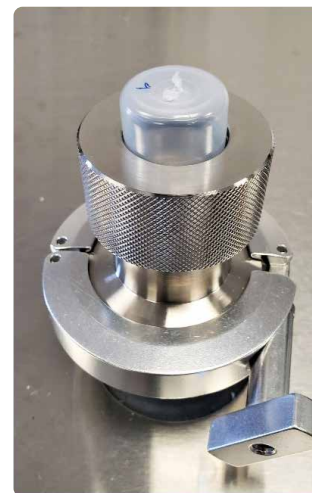
Bottle Vacuum test fixture with closure/neck under vacuum pressure
